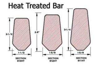
\* ITR Grouser Bars come in 10 foot lengths making it easy to inventory and cut to size as needed. Long grouser bars are also used in other applications including scraper flights, rock crusher liners, grizzlies, grader edges and are used for other applications requiring strength and abraison resistance.
